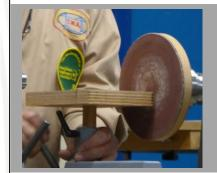
John continued the demo with a brief description of tool sharpening using a disc and 120 Rhino grit. This is especially quick and useful for skews and scrapers. He went on to show how he had made a jig for a medium sized router and demonstrated how to use the indexer to rout precise
