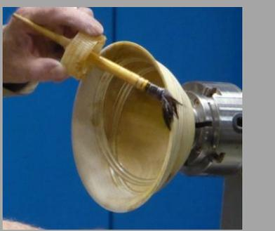
Was able to complete and polish the exterior and went on to show us the hollowing and finishing. After removal of the spigot he had a respectable bowl with intersecting rings.
