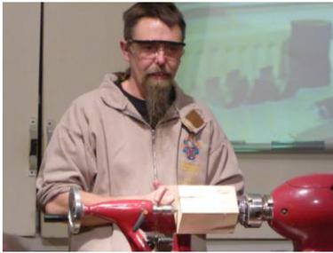
Andy braved some chilly conditions to come and demonstrate on Teesside so early in the year. He quickly ran us through procedures for hollowing, beginning with roughing to round, squaring ends and then creating chucking points. He began the hollowing by boring with a Forstner bit which he also showed us how to sharpen using a diamond 'credit card'.
