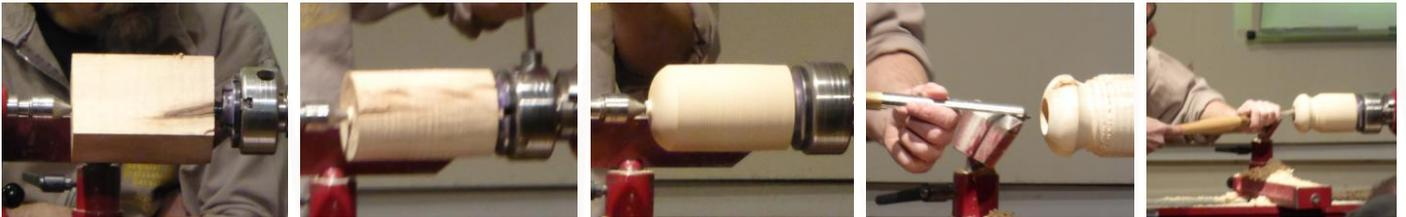
Whilst hollowing, Andy gave some useful tips about clearing enough space to allow a full reach across, and preferable around the end of the lathe bed to allow full access to the internal cut. He finished the hollowing with a scraper. When the first form was complete we took a break. After the break Andy repeated the techniques with a slightly larger form and went on to demonstrate some texturing.
