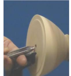
He turned the bowl with the thickness tapering toward the base so that the carved tree would be thicker at the bottom where the trunk and boughs are. The thickness would also give a natural seat to the bowl which he tested before deciding where to put the tree. Richard used his own special jaws for reversing the bowl, cutting a custom groove in the wooden jaws to fit the bowl he was making.
